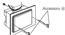
4. Lower the removal tool toward the bottom, and pull out the unit halfway while pressing towards the inside.
