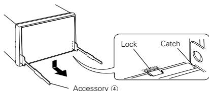
2. When the lower level is removed, remove the upper two locations.
